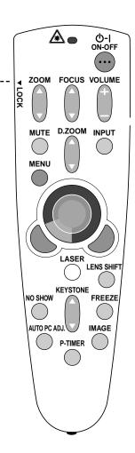
This Remote Control Unit emits a laser beam as laser pointer function from Laser Light Window. When LASER button is pressed, laser light goes on. And when LASER button is being pressed for more than 1 minute or LASER button is released, light goes off. LASER POINTER INDICATOR lights RED and Laser is emitted with RED light to indicate laser beam is being emitted.
